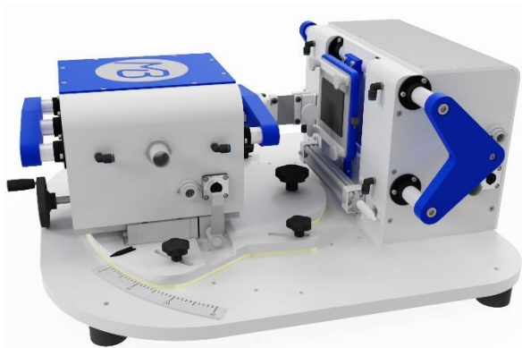
Figure 9: Plug-in connections for all supply lines directly at the test bench enable easy relocation and integration of the test bench into a climate chamber
