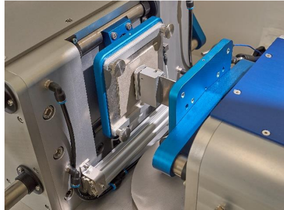
Figure 8: Sample holder with leaf spring and integrated sensors for testing in accordance with VDA 230-206
