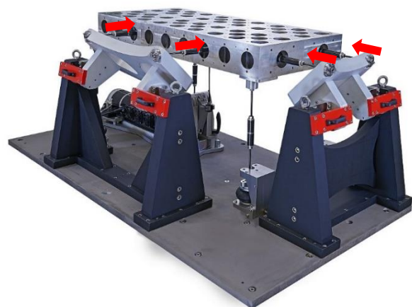
Figure 3: Guide and transmission arms ensure synchronous excitation and guidance of the magnesium table.
