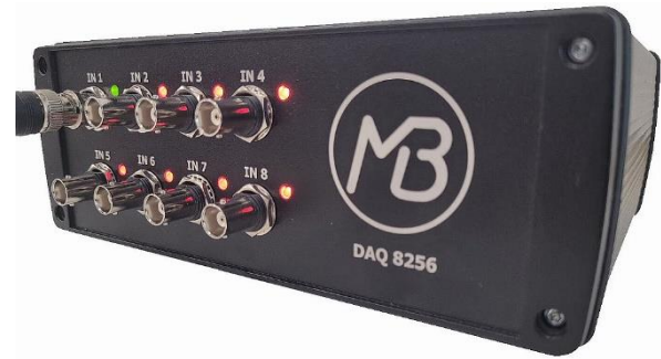
Figure 1: Status LEDs for each analogue input indicate whether the input is open, the IEPE sensor power supply is activated, or the input channel is overloaded.
