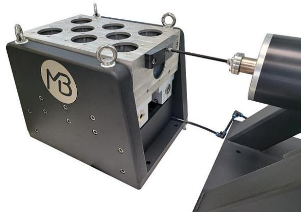
Picture 9: Horizontal Moving Table for ALPHA shakers
