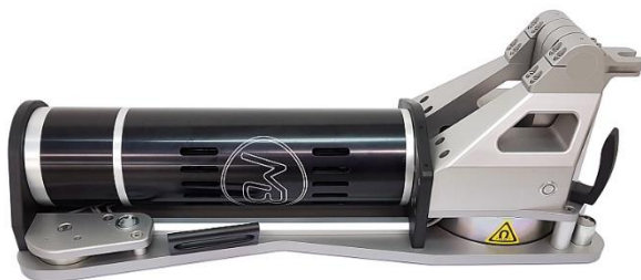
Picture 10: ALPHA 2025 in movable MLB-Base („Movable Lever Base“) with integrated 2:1 lever arm and electromagnets for electromagnetic clamping
