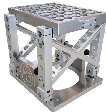
Picture 9: Horizontal Moving Table for ALPHA shakers
