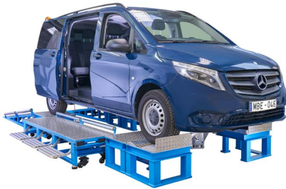
Figure 2: Vehicle stand and drive-on ramps. Mobile drive-over bridges with integrated, foldable steps facilitate safe entry and exit into the vehicle.
