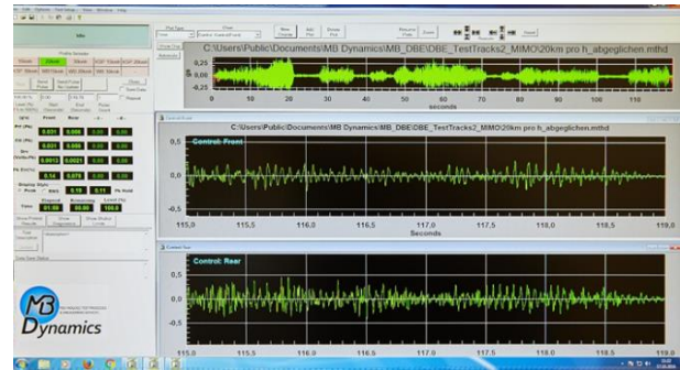
Figure 1: MB Millenium vibration control system for closed-loop control and monitoring of up to four vibration exciters enables reproducible simulation of a wide range of test tracks
