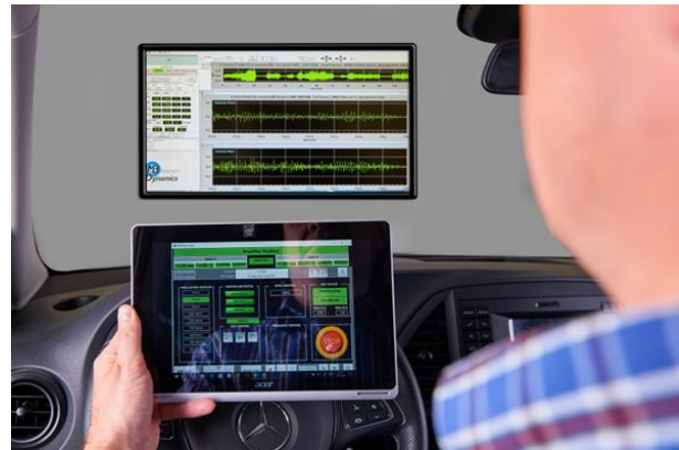
Figure 4: Remote tablet with simplified user interface enables selection of excitation profiles and operation of the test bench from inside the vehicle
