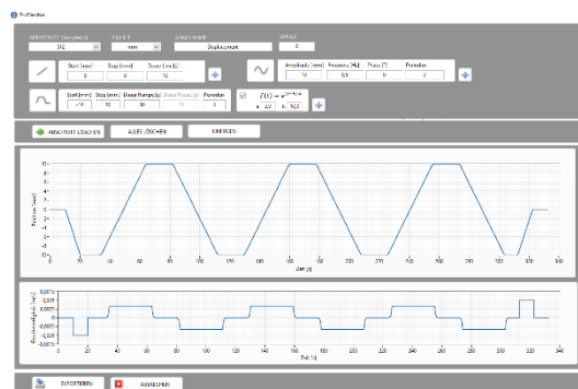
Figure 4: Definition of a ramp-shaped motion profile
