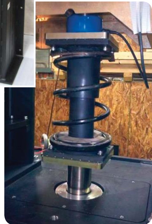
SUSPENSION RIG ASSEMBLY WITH COIL SPRING
